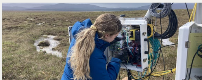
Research assistant with the VistaMilk SFI Research Centre, Aoife Jones, sets up an eddy covariance tower in a bog in Sligo.
